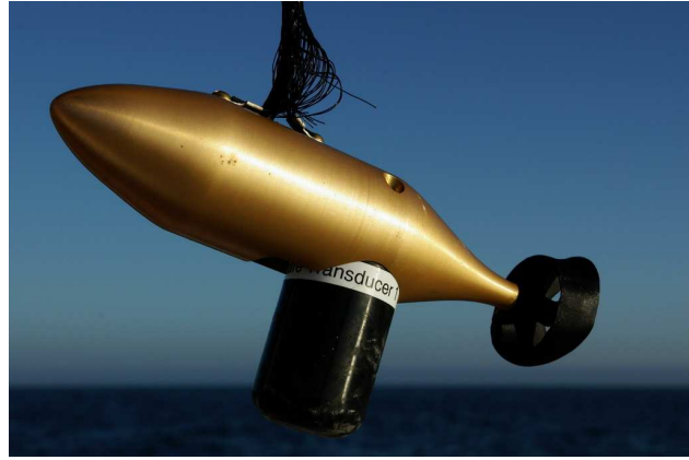
(b) Towfish with modem transducer
