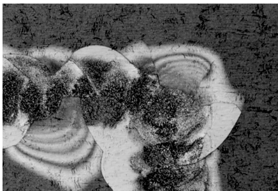
FIGURE 6: Photography of a top scribe of the structure PI / Al-ZnO / n-i-p / ZnO
