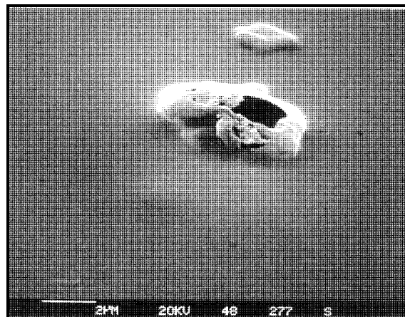
Figure 2: SEM micrograph of surface defect of a polyimide film
