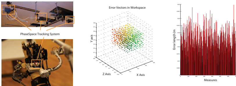
Figure 4.5: Results of the CyberTrack calibration procedure, compared to motion capture data.
