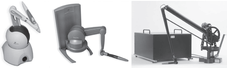
Figure 2.3: The Phantom® family. From left to right: Phantom Omni, Phantom Desktop and Phantom Premium.
