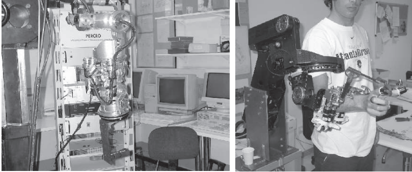
Figure 2.6: Two arm exoskeletons made at PERCRO, Scuola Superiore Sant'Anna, Italia . (Reproduced with Permission)
