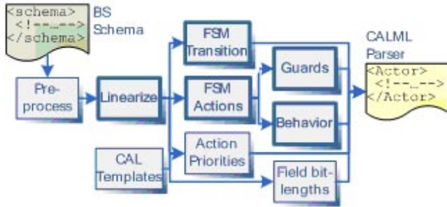
Fig. 7. The XSLT transformation process
