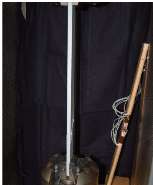
Fig. 1. 10° off-axis tensile experiment setup for in-plane shear strength
