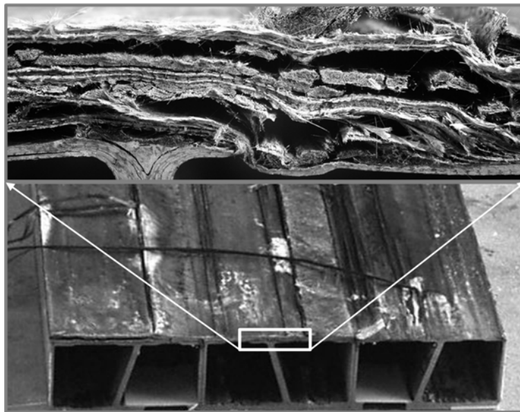
Fig. 1. Cross section of FRP profile after fire exposure
