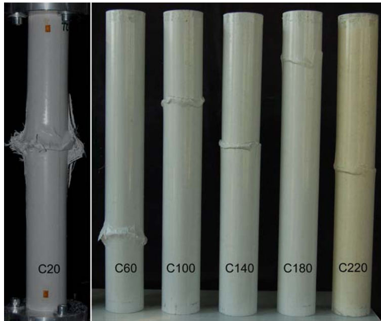
Fig. 8. Failure mode in compression experiments at different temperatures
