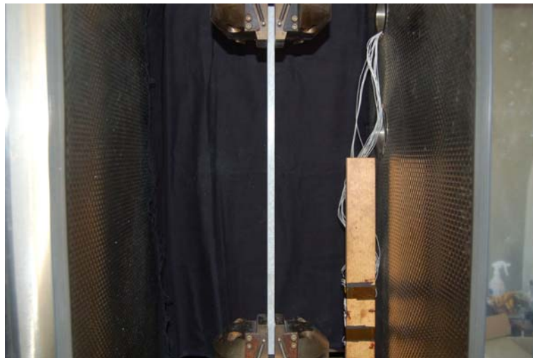
Fig. 7. Tensile experiment setup for tensile strength
