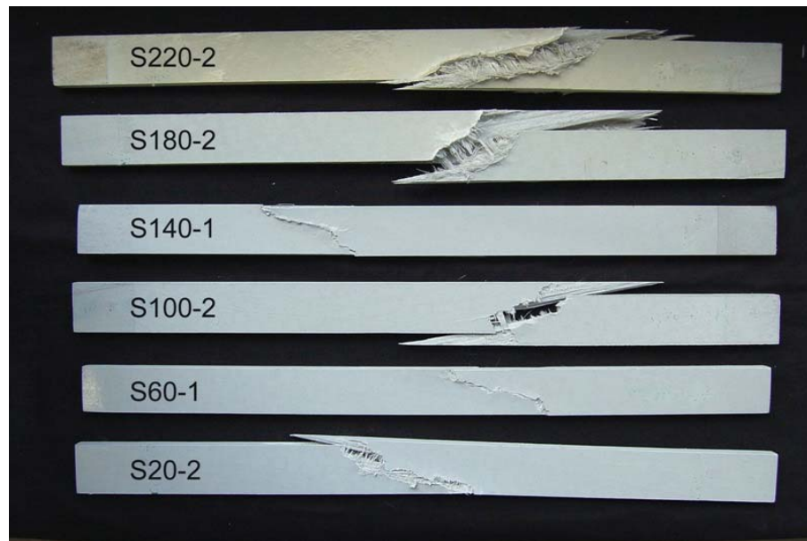
(l) Frontal view of typical damaged specimens
