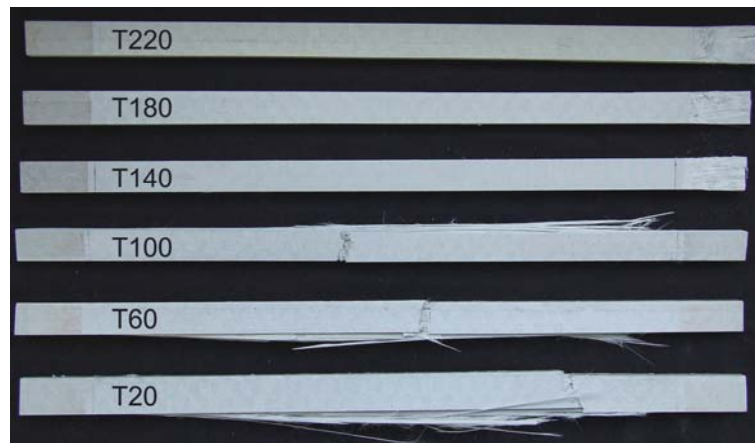
Fig. 4. Failure mode in tensile experiments at different temperatures
