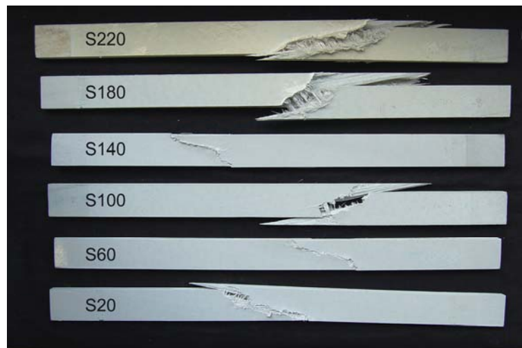
Fig. 2. Failure mode in 10^{\circ} off-axis tensile experiments at different temperatures
