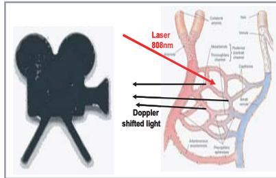
By using an 808nm laser as illumination, oxy- and deoxy-hemoglobin are sampled equally and so, by collecting the Doppler shifted light we obtain information on all the red cells moving in the illuminated tissue, hence we can visualize: Perfusion, Concentration of moving cells and their Speed distribution.
