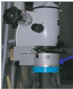
The LDI has been designed to fit beneath a standard surgical microscope and is non-invasive as it does not come into contact with the patient and is classified as laser class I.
