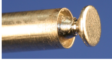
Figure 6.9: Modified Cutting Tip to Allow Measurements
