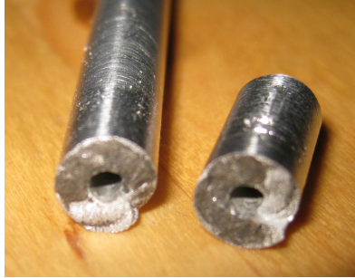
Figure 6.6: Second Prototype Cracked Transmission
