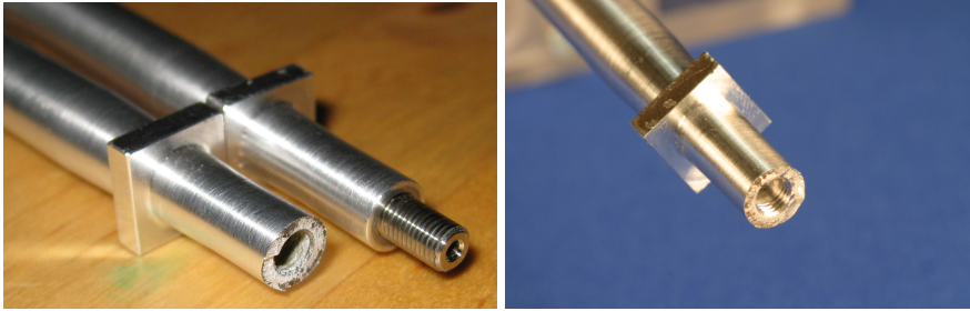
Figure 6.4: Second Prototype Cracked Parts
