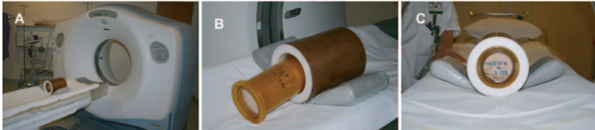
Fig. 8.3 Illustration of the third-generation XRCT scanner used at the service of radiodiagnostic and interventional radiology, CHUV, Lausanne. Although XRCT techniques are nowadays widely used in material sciences and designed for high-resolution imaging, the sample size is still a limiting factor. For samples corresponding to geotechnical rock cores dimensions (76-85 mm diameter and 150-170 mm length) the medical XRCT remains a fast and accurate technique for indirect imaging of whole rock structures even though limited to an effective resolution of 0.5 mm. A) General view of the CT scanner, X-ray tube and table. B) A geotechnical rock core placed in a rubber membrane as used for triaxial mechanical testing. The membrane is then placed into a PVC cylinder covered by a thin copper sheet in order to prevent beam hardening effects. C) End positioning of the sample at the middle of the CT gantry just before completion of the scan. For more details on the acquisition technique, see sections 8.3.2-4 .
