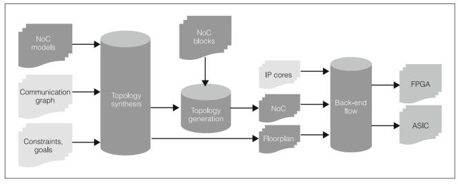
Figure 1. A design flow for network-on-chip (NoC) design. (Courtesy of iNOCs.)
