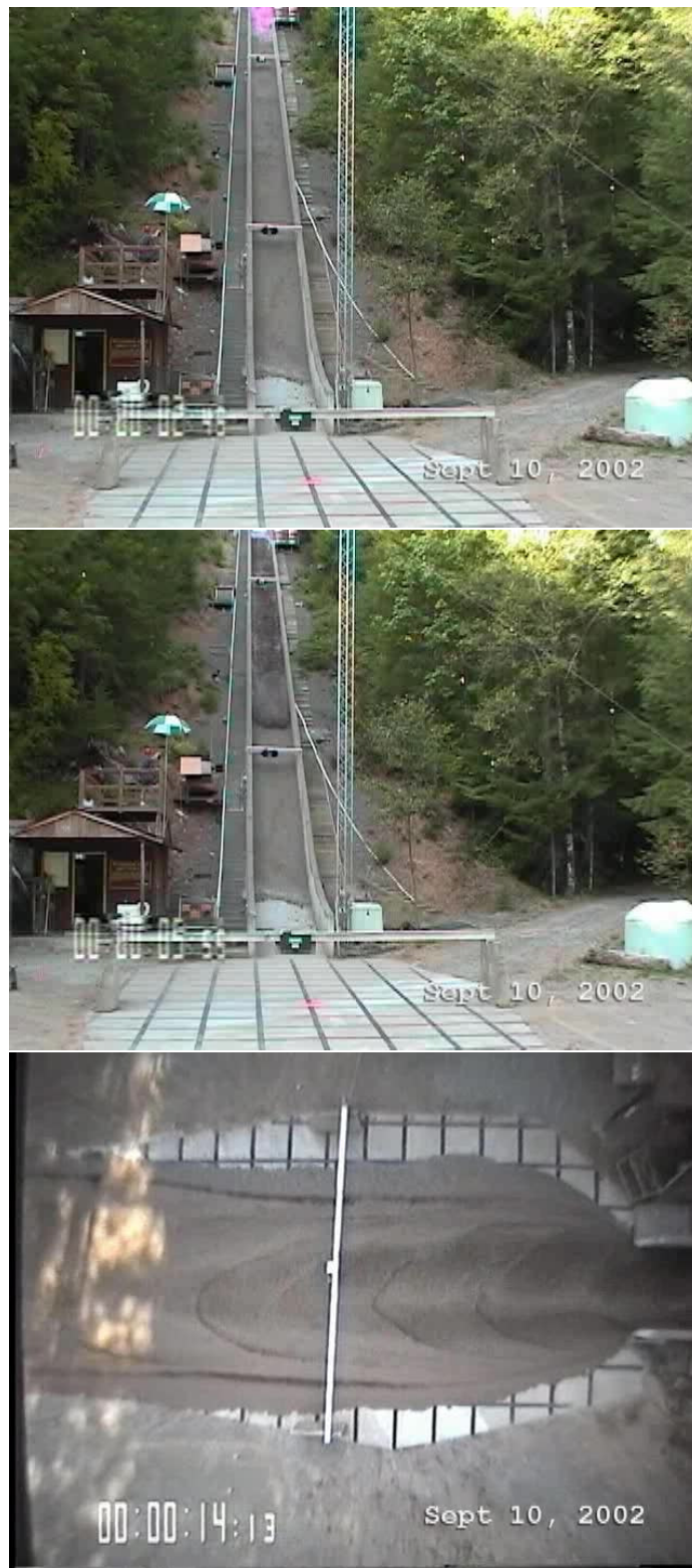
Figure 4.12: Roll-waves in water flood over erodible sediment bed, observed in the experiments at the USGS Debris-Flow Flume (Logan and Iverson, 2007).
