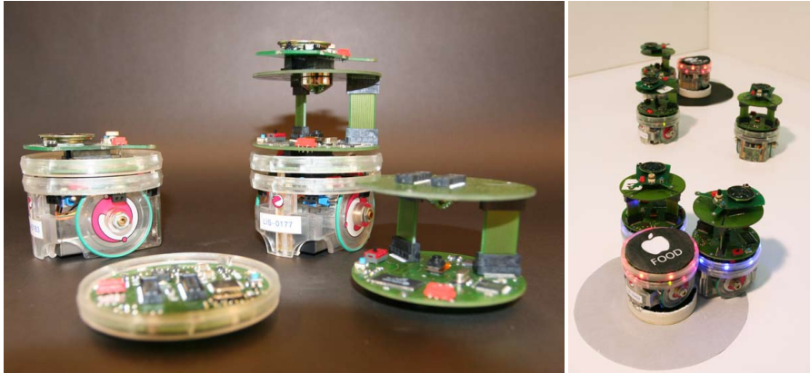
Fig. 1. Left: The e-puck robot is equipped with an omni-directional camera turret and an LED light turret used to emit blue light. It can thus be used to carry out experiments similar to that described in Chapter ?? . Right: A replicate of the experiment in Chapter ?? . Robots explore the arena containing food (bottom left) and poison (top right) objects emitting red light. Robots that have detected the food light up in blue to attract others.
