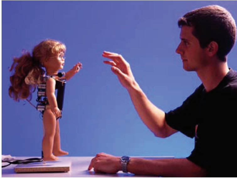
Figure 2.1: A Pocket PC mounted with a FlyCam Camera tracks the motion of the user and sends commands to the micro controllers and servos of Robota, so that it can imitate the motion of the head and arms of a user.
