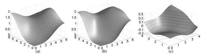
Fig. 6. Error kernels for the second order hex-spline  $\eta_2$ : (a)  $E_{\rm int}(\omega)$  for interpolation (with no prefilter); (b)  $E(\omega)$  for quasi-interpolation using the FIR prefilter proposed in Table I; (c) the difference  $E-E_{\rm int}$ , which confirms the better approximation quality when using quasi-interpolation.
