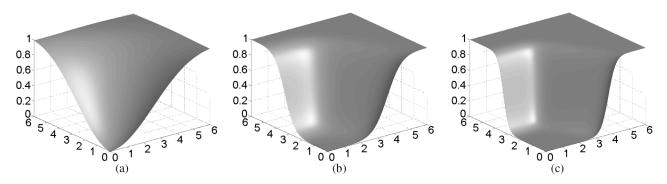
Fig. 5. Error kernel  $E_{\min}$  for (a) first-order hex-spline  $\eta_1$ , (b) second-order hex-spline  $\eta_2$ , (c) fourth-order box-spline  $\chi_4$ . As the order increases, the error kernel vanishes more and more in the hexagonal Nyquist region.
