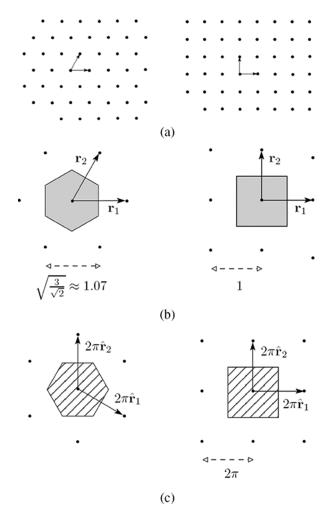
Fig. 1. (a) Hexagonal lattice of the first type  $\Lambda_{\rm hex}$  and the orthogonal lattice  $\Lambda_{\rm orth}$ . (b) Their respective Voronoi cells and (c) the corresponding natural Nyquist regions in the Fourier domain. Note that the reciprocal lattice of  $\Lambda_{\rm hex}$  is a hexagonal lattice of the second type.
