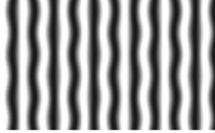
Fig.3 Intensity image of projected fringes with carrier frequency f_0=10.5
