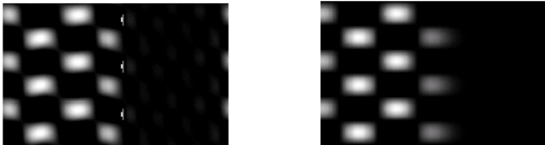
Fig.14 Height demodulated from Fig. 12(b) using (a) Fourier transform and (b) Wavelet Transform analysis
