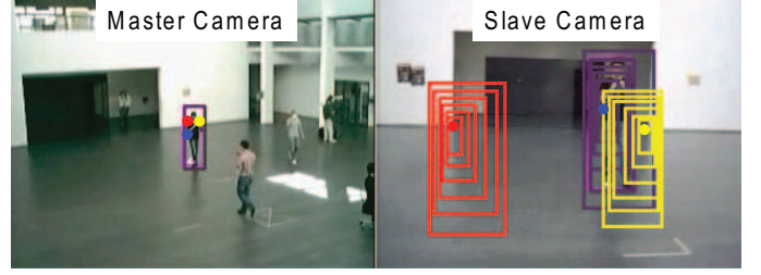
Figure 4: Illustration of an object described by 3 IP. The most similar IPs in the slave camera leads to 3*6 candidate regions only
