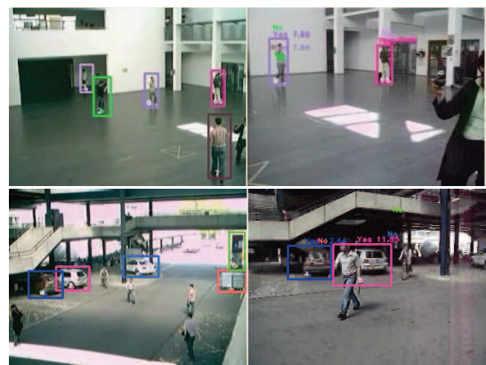
Figure 1: Left column: objects of interest highlighted in a fixed (master) camera. Right column: Corresponding objects detected and tracked in a mobile (slave) camera by our proposed approach
