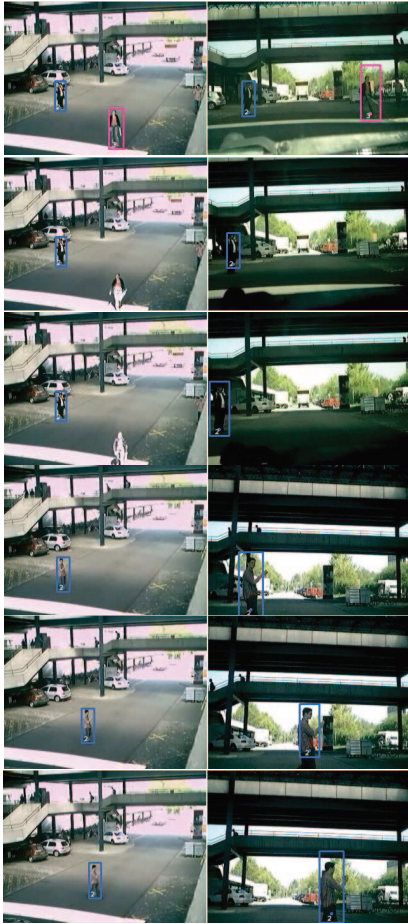
Figure 21: First column: objects detected by a master. Second column: corresponding objects detected with the slave given only the observation from the master.
