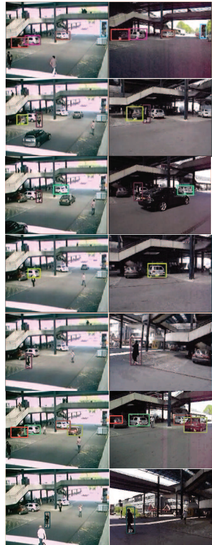
Figure 20: Examples of correctly detected and matched objects in outdoor scene. 1st column: objects of interest seen in a master. 2nd column: corresponding detected objects in a slave
