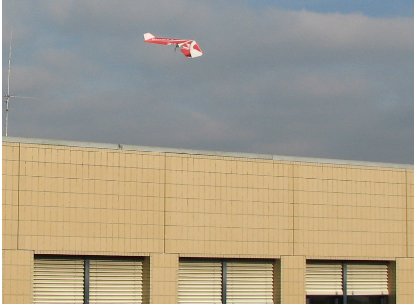
Figure 7: The 300-gram flying wing testbed that will be used for optic-flow-based navigation in cluttered outdoor environments.
