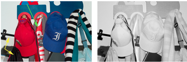
Figure 4. A scene with colourful objects. Note that the red and white scarf pattern (middle of the image, green arrow) disappear in the near-IR. On the other hand, the two black objects (left side of the image, yellow arrows) have a very different near-IR response.
