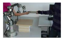
Fig. 1. In a scenario used for collecting data and preliminary experiments, a robotic arm (KATANA from Neuronics) assists a human collaborator to transport an object. The human wears a motion suit that captures motion of her joints, thus a robot knows the posture of the human arm at each time step. Another person kinesthetically guides the robot demonstrating its part of the task.
