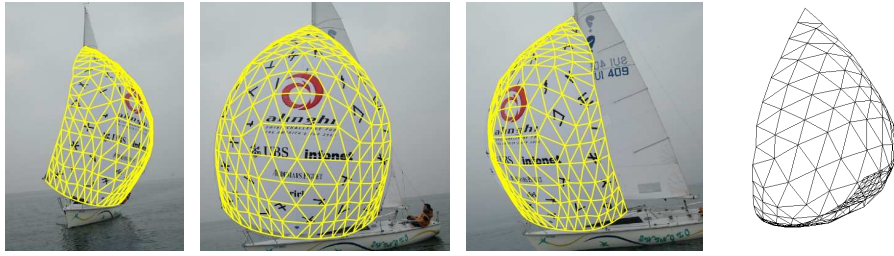
Figure 5.15: 3D model of the spinnaker overlaid on the three images used to compute its reference shape and texture. In each image, we specified 10 correspondences with a CAD model of the spinnaker and used them, along with automatically detected silhouettes, to deform it. We assume that the spinnaker did not deform in these images because they were taken in quick succession by a chase-boat.
