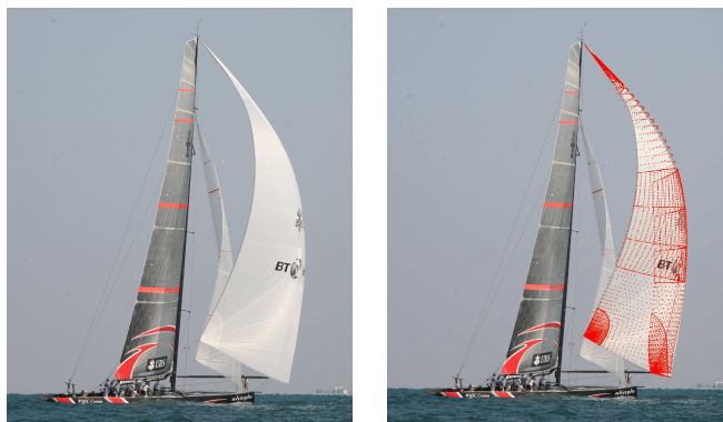
Figure 8.1: Some of our techniques have been used in a software that computes the shape of the spinnaker of the swiss sailing team Alinghi.
