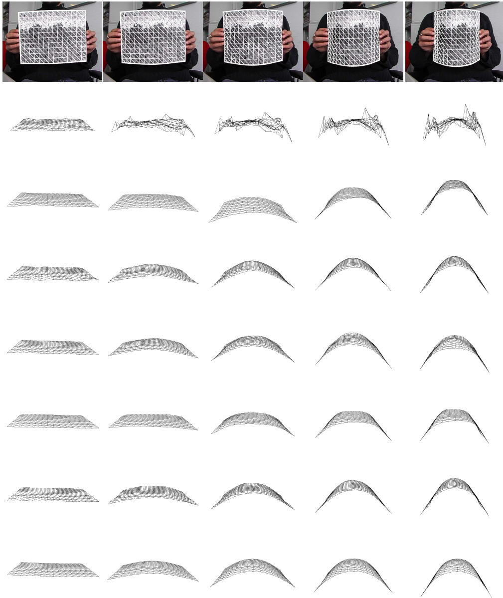
Figure 7.15: We compared our methods on a real video of a deforming sheet of cardboard. In order to texture it, and thus make it usable for correspondences-based techniques, we stuck a piece of paper on the cardboard. Since cardboard is more rigid, its behavior remains unchanged. Top row: Reprojection of the results obtained with the linear local model. Next rows: Results obtained, from top to bottom, with linear motion model, convex optimization, linear global model by tracking and in closed-form, non-linear local models, linear local models by tracking and in closed form.
