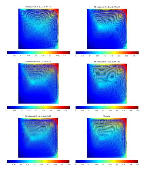
Fig. 3. Streamlines at Grashof number  $Gr = 10^5$ , Prandtl number Pr = 1, and aspect ratio A = 1: streamlines of the reduced basis solution for N = 2, 3, 4, 5, 6 and of the reference finite element solution.
