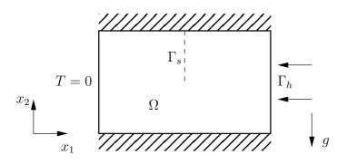
Fig. 1. A closed cavity. On the left the temperature is constant, on the right the heat flux is constant, and the top and the bottom of the cavity are insulated.
