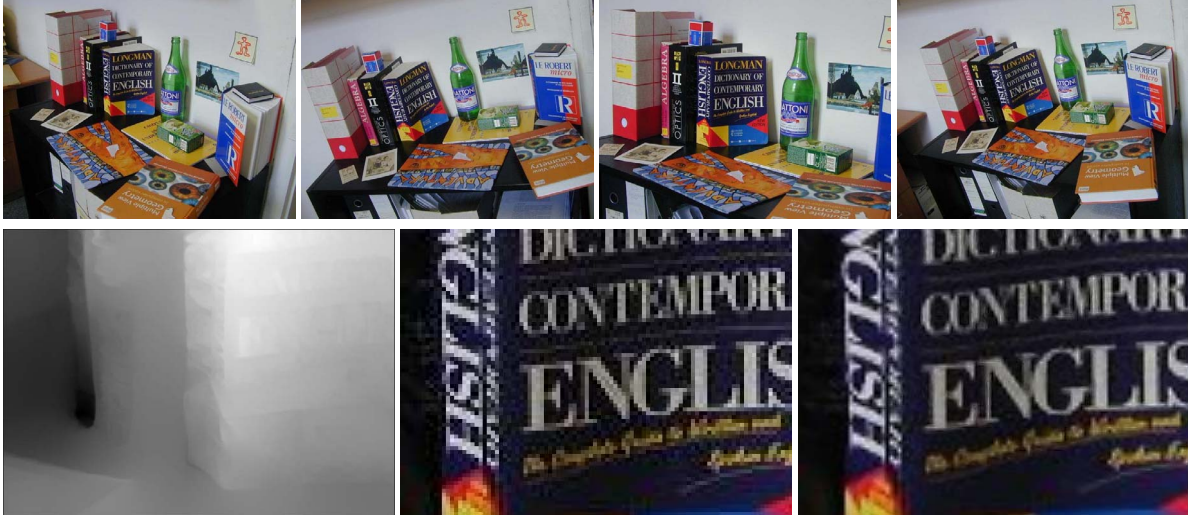
Figure 1: Bookshelf scene: The top row shows the 4 original input images. In this experiment, we zoomed in a virtual camera on the first image ( \mathcal{I}_1 ), to visualize the integration effects of \mathcal{I}^* . The second row displays the output of the algorithm. Here, the 1 th image is the depth map \mathcal{D} computed from the new camera position. The last 2 images show a detail of \mathcal{I}_1 and \mathcal{I}^* , respectively. By integrating the information of all 4 views, the discretization errors in \mathcal{I}_1 have largely disappeared.
