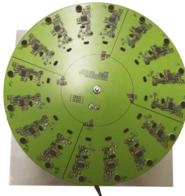
Figure 2. The array of the sixteen microphones (the view from above).
