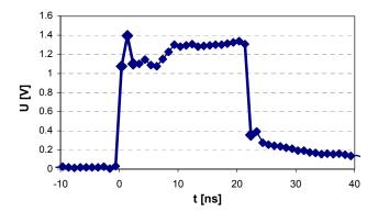
Fig. 3. Real electrical pulse used to simulate and experimentally test the effect of chirp, presenting an overshoot on the leading edge. Typical rise and fall times are 1 ns.
