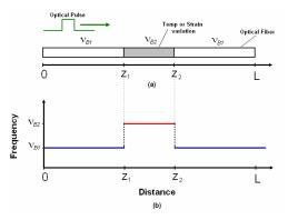
Fig. 2. a) Experimental configuration to test the effect of the modulator chirp;  $v_{Bl}$  represents the natural Brillouin frequency of fiber and is the Brillouin frequency of a singular section (e.g. the temperature or the strain on the fiber is changed). b) Corresponding distribution of the Brillouin shift.
