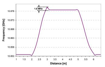
Fig. 4. Calculated Brillouin frequency as a function of position for an irregular trapezoidal pulse, simulated for a 0.1 rad/s chirp value. Pulse characteristics are: 10 ns width, 1.5 ns rise/fall time, overshoot is 15% over the pulse top.
