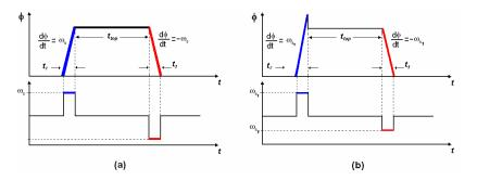
Fig. 1. Phase change (top) during the pulse forming using an electro-optic modulator and corresponding instantaneous frequency (bottom): a) trapezoidal pulse shape. b) irregular pulse with overshoot.
