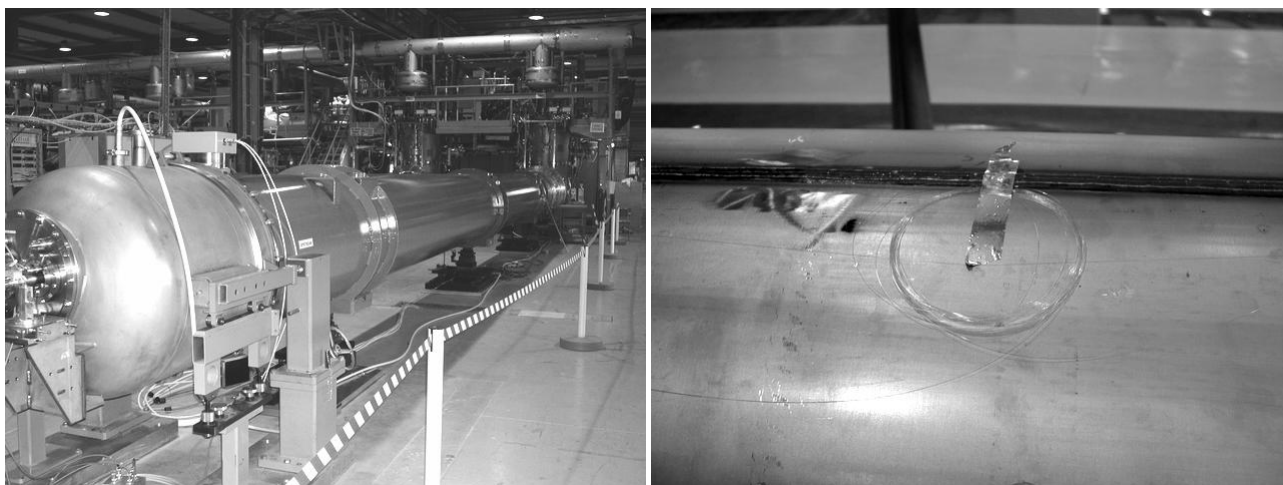
Fig.4 Magnet of the future CERN large hadron collider (left) and installed fiber for probing temperature on the wall of the liquid helium inner vessel (right).
