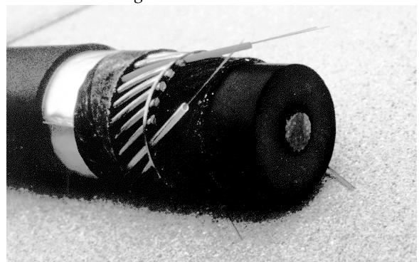
Fig. 14 High-voltage 60kV cable with bundled fibers for temperature monitoring.
