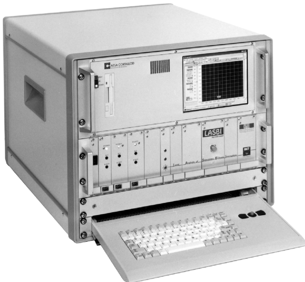
The Brillouin distributed fiber sensor LASBI 9800.
