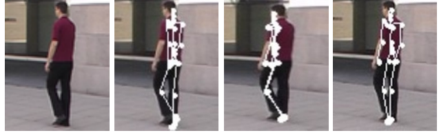
Figure 3. Refinement process. The images are from left to right the input image, the initialization given by the interpolation process, the refinement obtained without using the background generation, and finally the refinement obtained as proposed. Whole parts of the body can be missed when the background is not exploited.
