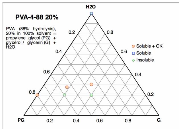
**Fig. 2.** PVA-4-88 20% in 100% PG+G+H<sub>2</sub>O.
