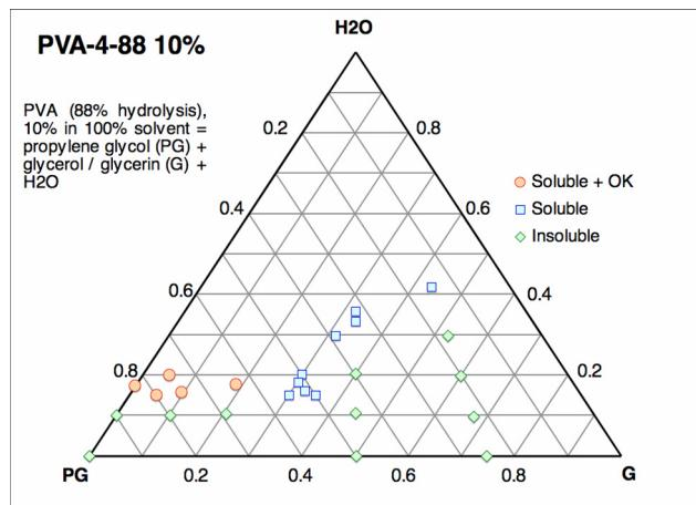
**Fig. 1.** PVA-4-88 10% in 100% PG+G+H<sub>2</sub>O.
