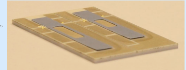
Capacitive microforce sensors (dielectric cantilever) [1,2]
