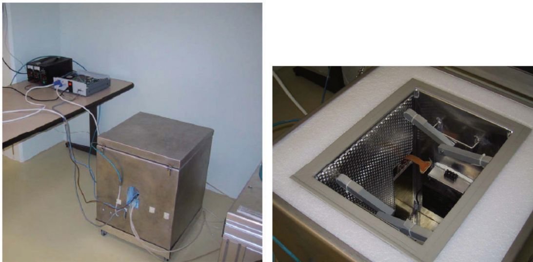
Figure 4.9: Burn-in and temperature cycling box at CERN. All modules have been tested in a thermally isolated box with temperature control built by the University of Santiago. The measurements include IV-curves reading and the leakage current monitoring during the temperature cycling. Readout of the modules using the internally provided test pulses has also been performed during this temperature cycling in order to spot broken (open/shorted) channels.
