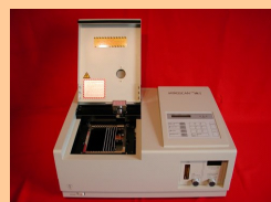
Fig 2 : IATROSCAN device for determining the bitumen generic composition
