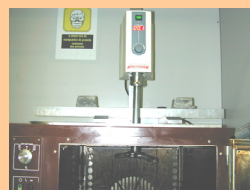
Fig 1 : specimens mounted on a high speed mixer inside and oven
