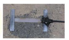
3 LVDT sensors for the measurement of surface deflection
