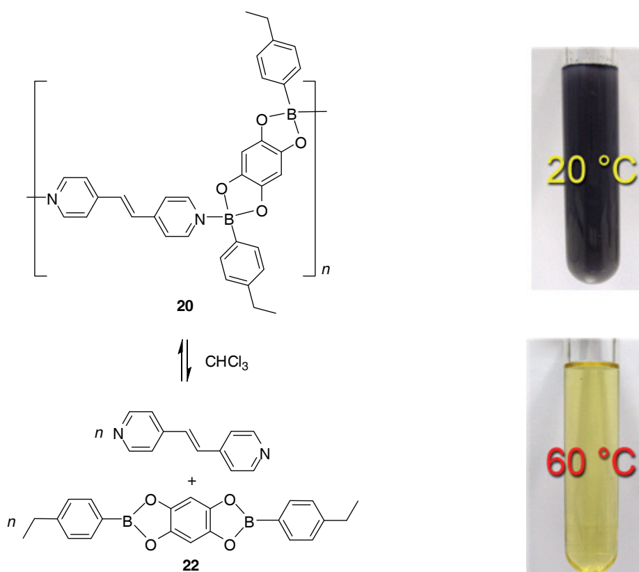
Scheme 4.2: Equilibrium (in \text{CHCl}_3 ) between polymer 20 and its constituents 22 and 1,2-bis(4-pyridyl)ethylene (left) and the color change observed upon heating (right).
