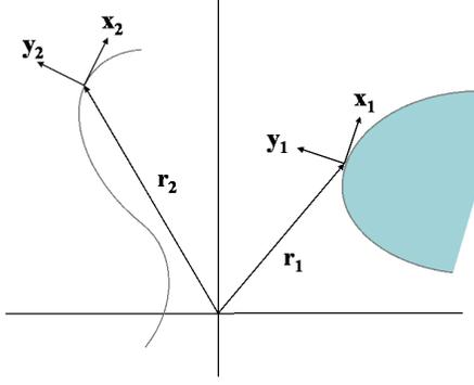
Fig. 1. Positions and frames for the trajectory of the moving vehicle ( $\mathbf{r}_2$ ,  $\mathbf{x}_2$ ,  $\mathbf{y}_2$ ) and for the closest point on the boundary curve ( $\mathbf{r}_1$ ,  $\mathbf{x}_1$ ,  $\mathbf{y}_1$ ).
