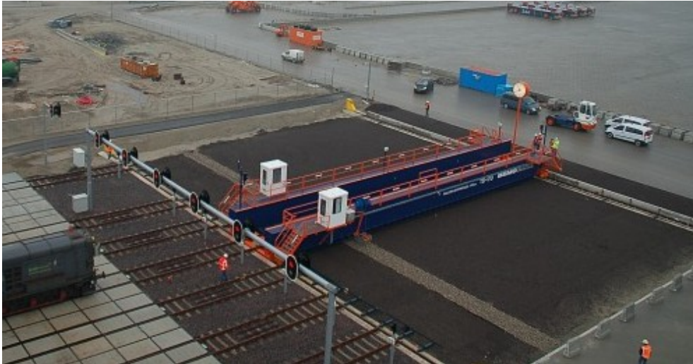
Figure 4 Example of a discontinuous way of changing tracks: a travelling platform in Rotterdam (NL) 1
