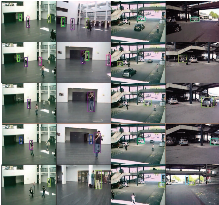
Fig. 11. Random Examples of the proposed system. 1st and 3rd column: objects of interest seen in fixed camera. 2nd and 4th column: corresponding detected objects in the mobile camera (output of the proposed approach)
