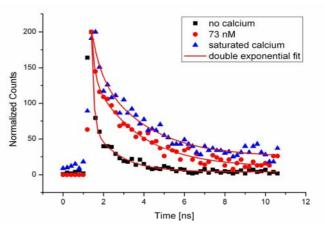
Fig. 1. Measured and numerically fitted fluorescence response of OGB-1 in the presence of various Calcium concentrations.
