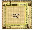
Fig. 3. Random access SPAD array realized in 0.8µm CMOS technology.
