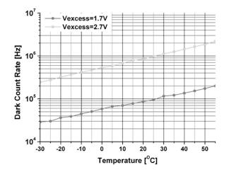
Fig. 8. DCR dependence on temperature.
