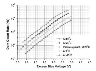
Fig. 9. Dark count rate (DCR) as a function of excess bias voltage at four temperatures. Temperatures are set with an uncertainty of  $\pm 2$  °C.
