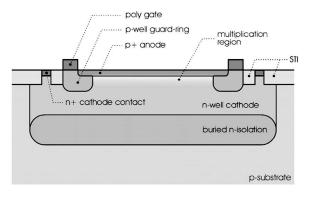
Fig. 1. SPAD cross-section: p+ anode within n-well cathode (not to scale).
