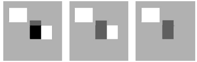
Fig. 2. A synthetic image (left) and the output of the 2D sieve algorithm after the minmax (middle) and maxmin (right) steps at a scale equivalent to the area of the black region.
