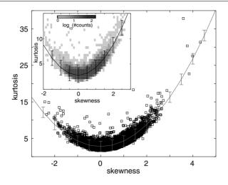
**Figure 2.** Kurtosis versus skewness computed for 8966 experimental signals. The fitting second order polynomial (solid grey line) is also plotted. (Inset) Joint probability of K and S for the experimental signals. On both graphs, the error bars correspond to the 95% confidence interval.
