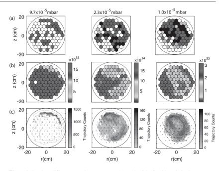
**Figure 1.** For three different neutral gas pressures: (*a*) result of the fit with optimized parameters. The color coding is the following: several PDF fit the experimental one (white), no PDF fit the experimental one (black), only one PDF fits the experimental one (soft gray), double-humped PDF (dark gray); (*b*) spectral energy contained in the mode and (*c*) statistics of structure trajectories.
