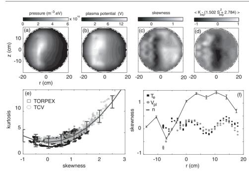
**Figure 4.** The 2D poloidal profiles of the time-averaged plasma pressure (*a*), plasma potential (*b*), density fluctuations skewness (*c*) and (*d*) difference between the experimental kurtosis and values from (2) (*e*). Kurtosis versus skewness for 2580 signals in the 'SOL-like configuration' in TORPEX (squares) and for 962 signals measured in the TCV SOL. (*f*) Radial profiles of the skewness estimated for *n*,  $T_e$  and  $V_{pl}$ .
