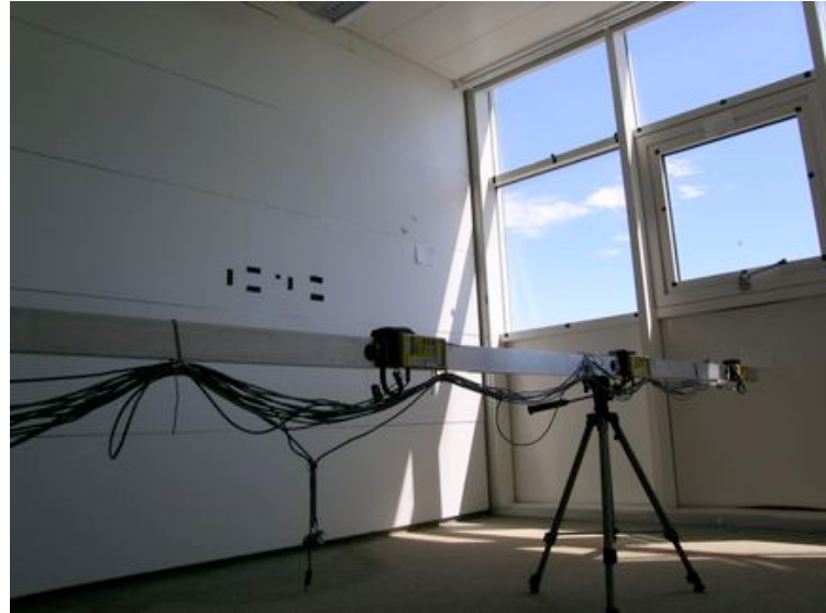
Fig. 3.35 → Internal view of the real building and calibrated BEHA 96408 sensors on a metal bar for indoor illuminance monitoring
