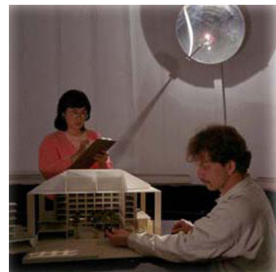
Fig 2.35 A sky dome at the Lawrence Berkeley National Laboratory, California (USA)
