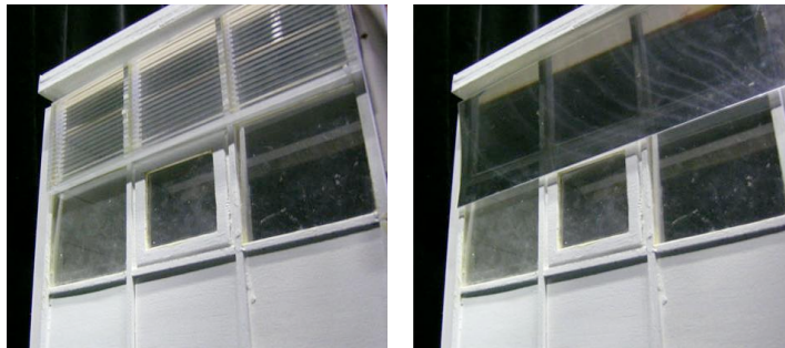
Fig. B 1 Scale model: CFS attached on the outside of the window
