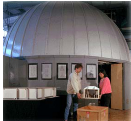
Fig 2.35 A sky dome at the Lawrence Berkeley National Laboratory, California (USA)
