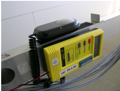
Fig. 3.34 Calibrated BEHA 96408 sensor for indoor illuminance monitoring
