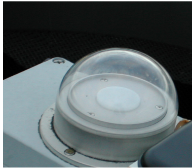
Fig. 3.28 A horizontal LMT/BAP30FCT for outdoor illuminance monitoring
