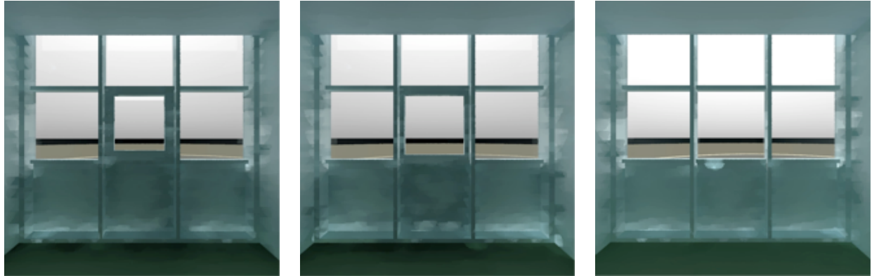
Fig. 5.8 Virtual models with both window frame and panel (left), only with window frame (centre) and without window frame nor window (right)
