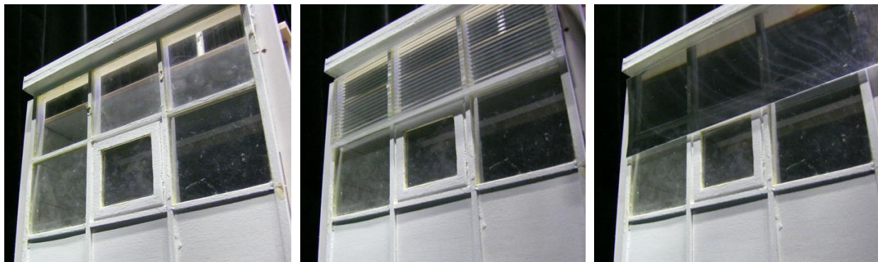
Fig. 3.52 Double glazing, Laser-cut panel and Prismatic film attached to the scale model's window
