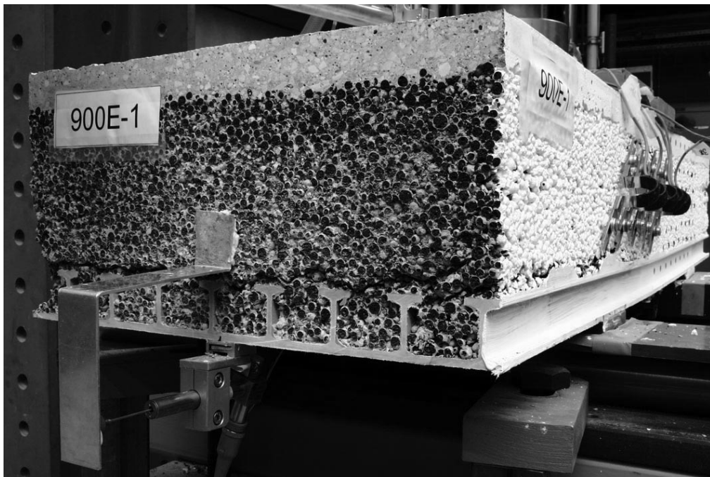
(b) Sheared LC-NC unity at north end, after experiment
