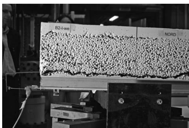
(b) Crack through eastern beam end
