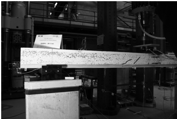
(c) Longer cracks through LC core at loads above 35 kN
