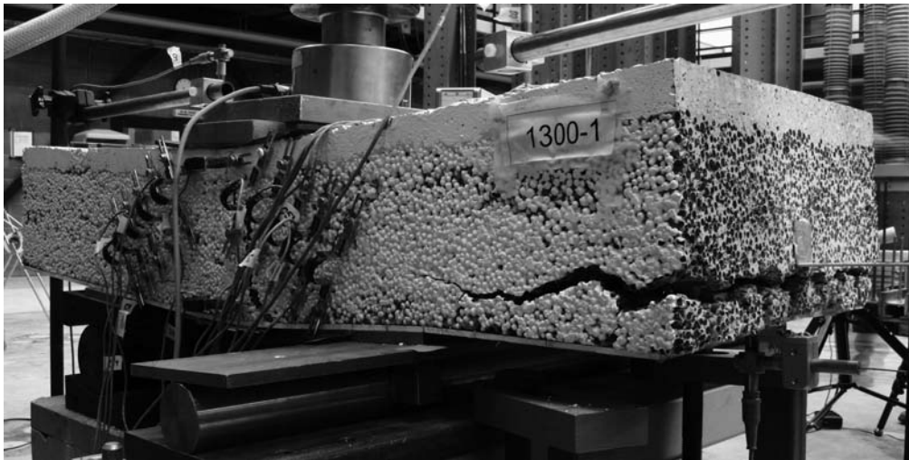
(a) Failed specimen east part
