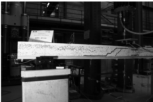
(e) Cracks through beam at 26.7 kN and 13.7 mm deflection
