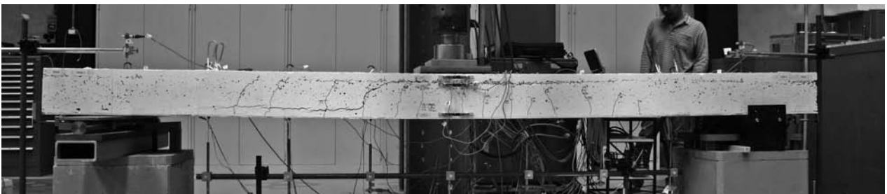
(b) Development of main crack at max load 35.0 kN
