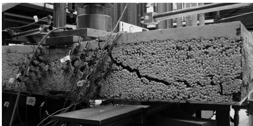
(c) Final crack development above all omega gages
