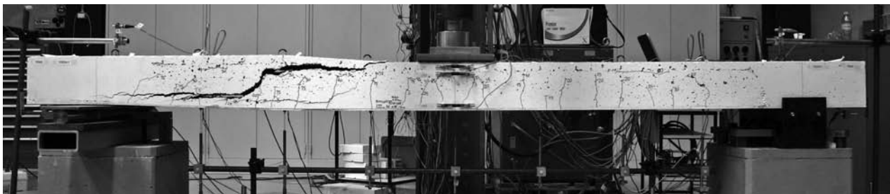
(e) Failed beam after experiment, still loaded
