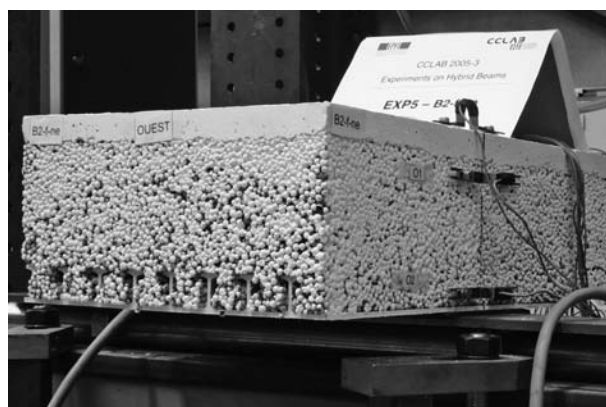
(c) LC being pushed out of GFRP profile at west end
