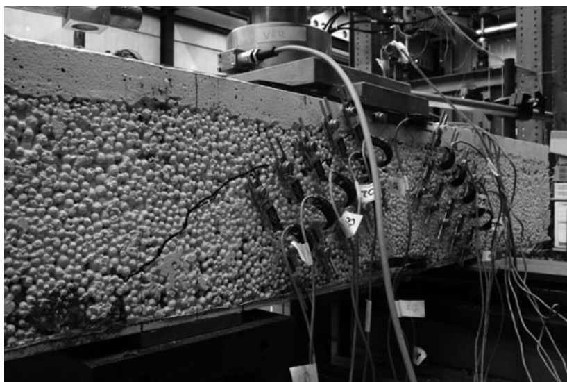
(b) At approximately 140 kN (post-peak) - crack development above O23 and O24
