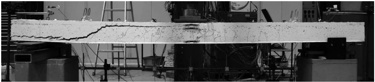
(c) Crack pattern at ultimate load
