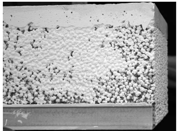
(f) LC being pushed out of GFRP profile at 8.3 kN (post-peak) at beam axis F
