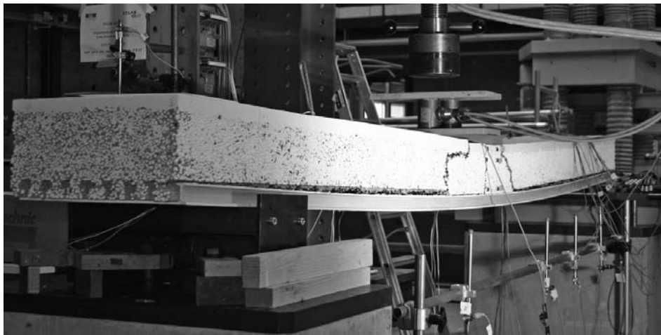
(b) View from north - unloaded failed beam after experiment
