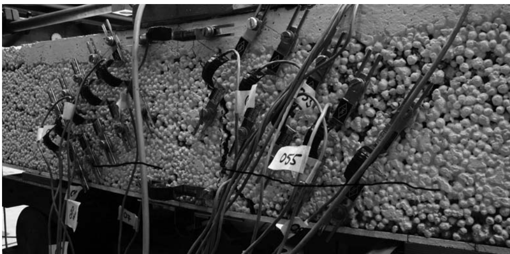
(d) Horizontal cracks on eastern part of specimen at 80 kN
