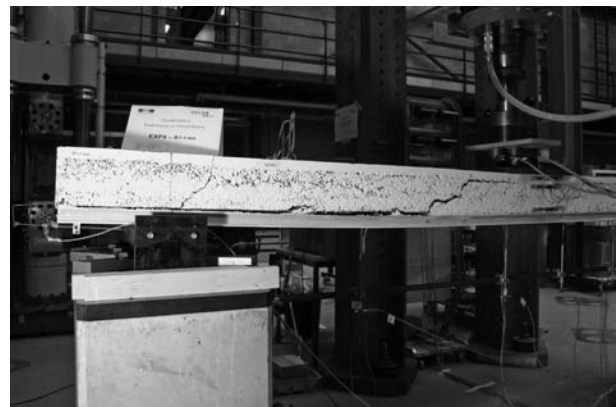
(f) Failed beam at 3.4 kN and 16.4 mm deflection
