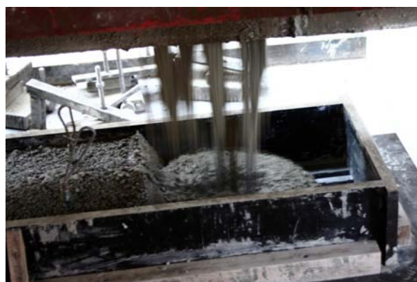
(b) NC casting of anchor blocks and upper layer
