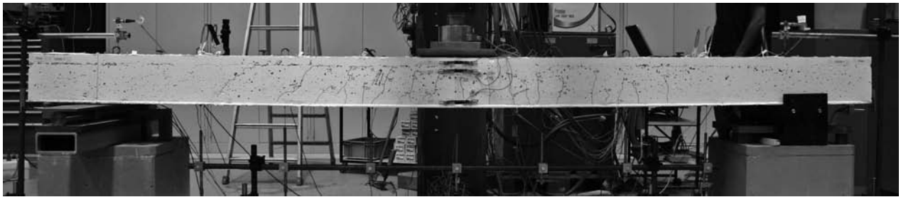
(b) Crack pattern at 30 kN - second load cycle
