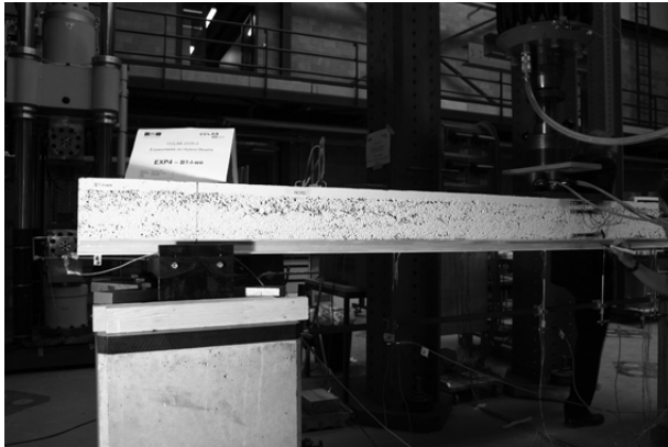
(a) First crack under loading plate at 20 kN
