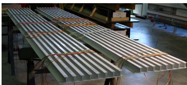
(b) Instrumented GFRP profiles
