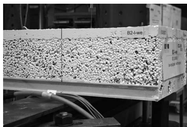
(c) Undamaged western beam end
