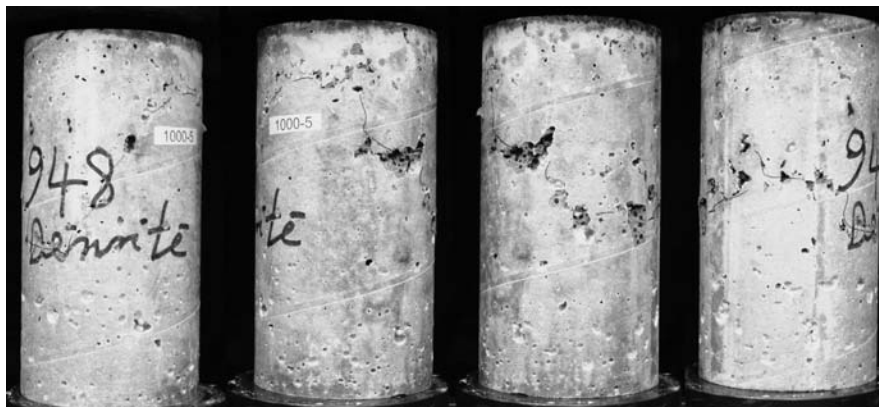
Figure B.8: Typical failed LC1000 cylinder.
