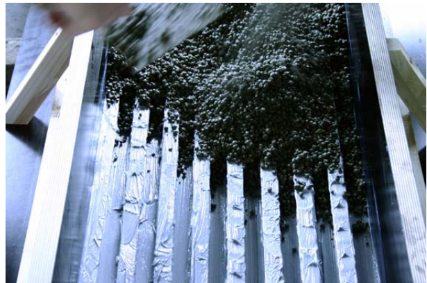
(b) LC casting onto fresh epoxy adhesive
