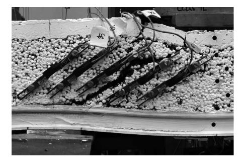
Figure 3.35: Typical failure of FRP T-upstands (beam 1300Es-2 at end of experiment).
