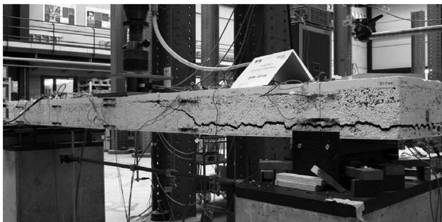
**Figure 3.15:** Failure pattern of bonded beam 1300E-2.
