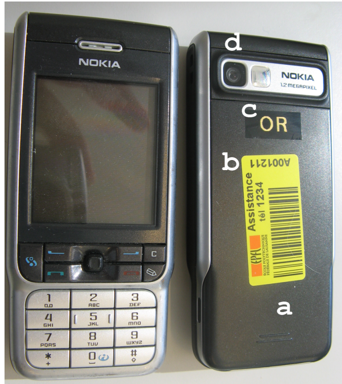
Figure 6-1: Example of phone used during the field trial. (a) phone serial number; (b) Bluetooth identifier; (c) color code added for the second field trial matching the mobile number of the phone in the address book ('OR' in French 'gold'); (d) camera lens
