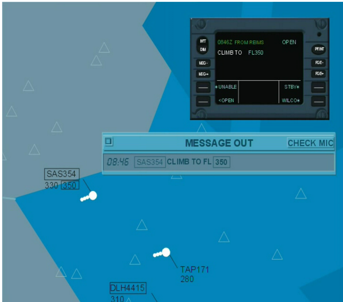
Figure 1-3: Interface of the HMI system. The traffic controller can click on the radar trace of a plane to activate textual communication with its pilots. The pilot sees the textual message appearing in a dedicated display represented in the top-right corner of the figure (© Eurocontrol 2008)
