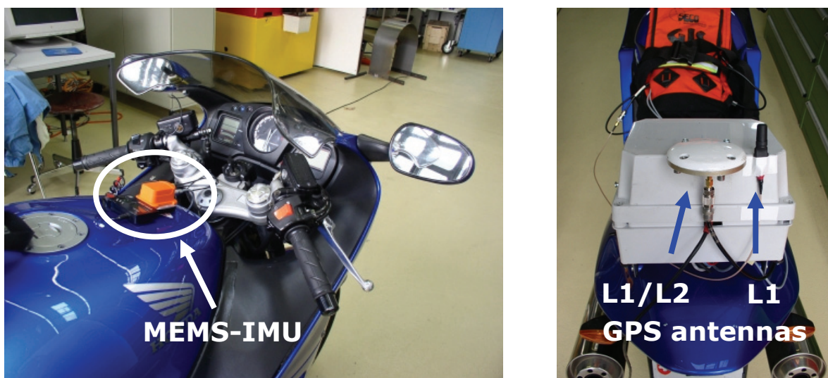
Figure 1 : GPS/MEMS-IMU system setup
