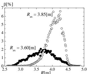
R[m] Fig.2 Normalized pressure profiles. Filled and open circles indicate the case of  $R_{\rm ax}=3.60[{\rm m}]$  and  $3.85[{\rm m}]$  respectively. The steep gradient is seen in  $R_{\rm ax}=3.85[{\rm m}]$ .
