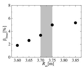
Fig.1 Magnetic axis ( $R_{ax}$ ) dependence of central beta ( $\beta_0$ ). Threshold is seen at between  $R_{ax}=3.7$ m and 3.75m. The  $\beta_0$  seems to be suppressed in inward shifted configuration ( $R_{ax}<3.7$ ).
