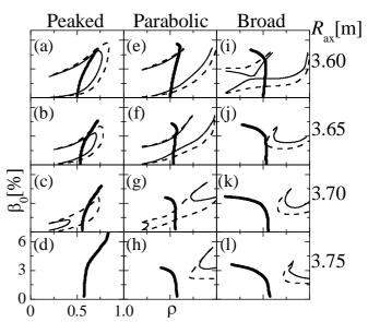
Fig.4 Contour lines of Mercier index and the position of  $\[ 1/2\pi = 1/2 \]$  surface in  $\[ \rho - \beta_0 \]$  space. Dashed and solid thin lines indicate  $\[ D_1 = 0 \]$  and 0.2 respectively. Bold solid lines correspond to the position of  $\[ 1/2\pi = 1/2 \]$ .
