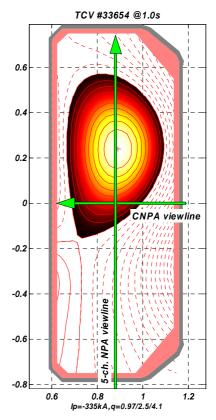
**FIGURE 1.** Poloidal cross section of the TCV Plasma configuration.
