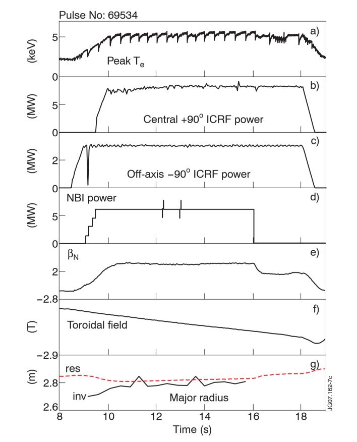
Figure 7. B<sub>T</sub> sweep. The optimum sawtooth stabilisation field in static conditions corresponds to the value reached here at 13 s, i.e. 2.85 T
