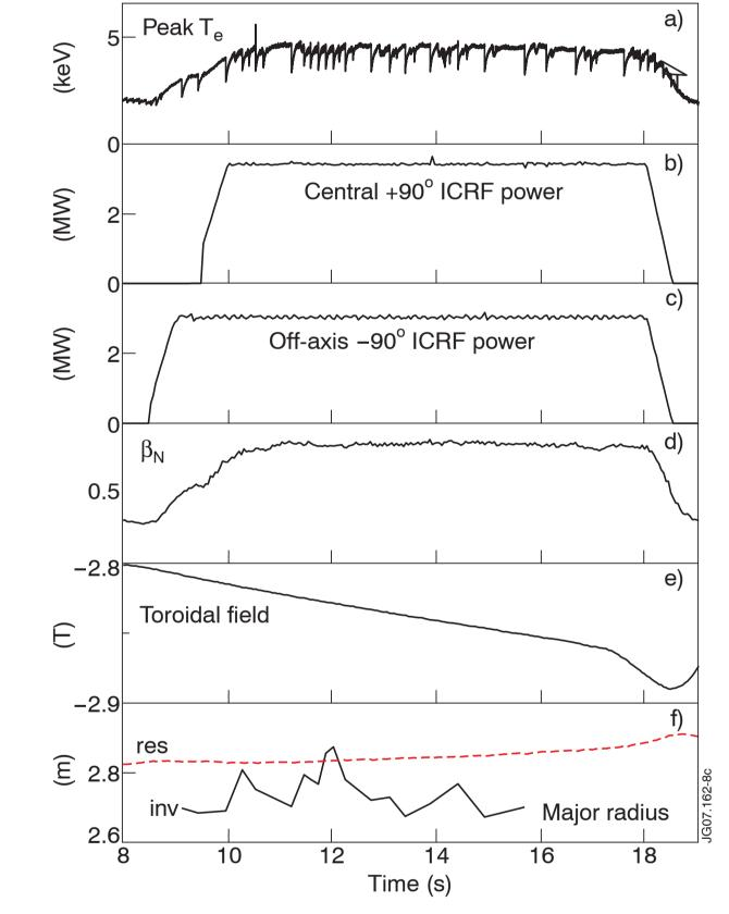
Figure 8. B<sub>T</sub> sweep with no NBI heating. The optimum sawtooth stabilisation field in static conditions corresponds to the value reached here at 12 s, i.e. 2.83 T
