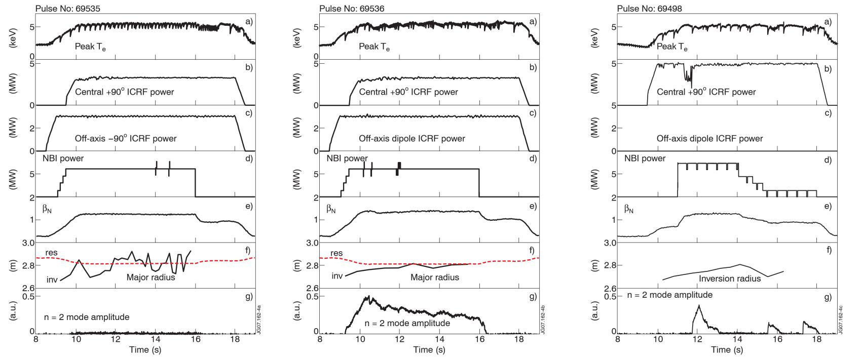
Figure 4. Discharges with off-axis counter-current propagating ICRF (left), off-axis dipole ICRF (middle), no off-axis heating (right)
